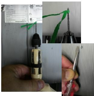
Next, take a hand-powered drill and insert a small bit into the chuck. Take a twist-wire from the kitchen, twist it onto the bit, and move it to about 1/8” from the tip. Position it on the mark where you want the hole, press slightly, and turn if necessary (*such as if you are penetrating sheet metal*). Penetrate only a little, in case there’s a refrigerant line inside. Enlarge the hole gently with a small screwdriver.
